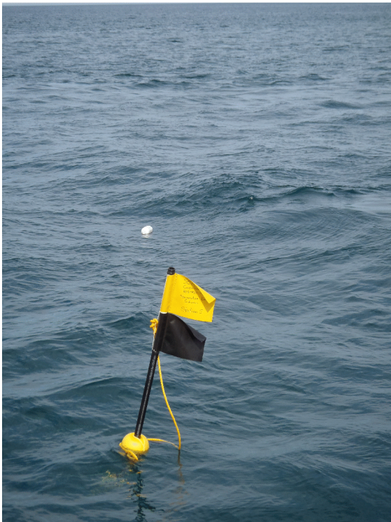
Figure 1: A spar and buoy are visible on the surface a short distance apart for each temperature monitoring location.
